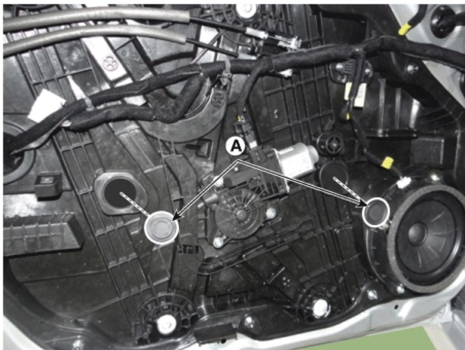
5. By operating the power window switch, pull down until the glass mounting bolt on plug hole is visible.
