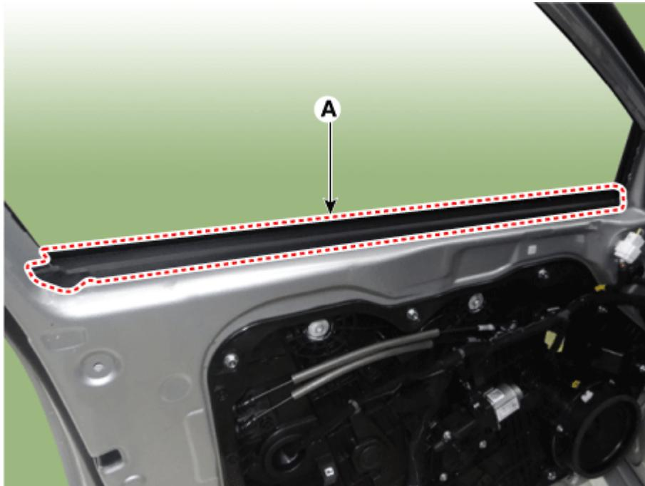
4. Remove the front door window glass mounting hole plug (A) from the door module.
